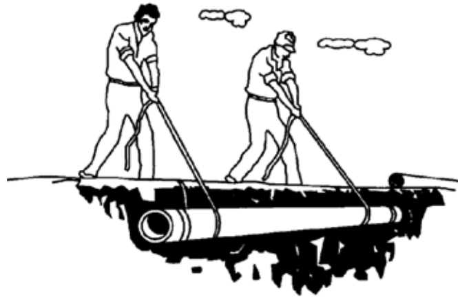
Figure 3: Lowering with ropes
